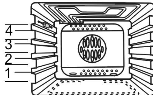
You also can bake on customary baking trays, which are to be placed on the grate. In this case baking trays out of black plate are recommended. These trays have a better heat conductivity, the baking time is reduced and energy can be saved.
